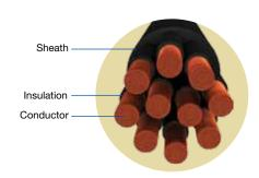
PVC Insulated Electric Cables Multicore Round
